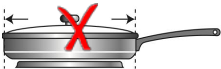
Pan/pot overhangs SmartBurner plate by more than 2.5 cm (1")
